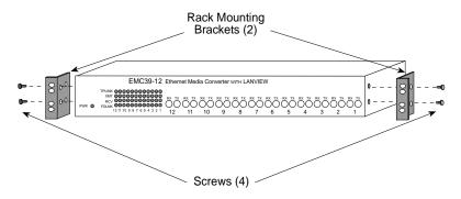
Figure 2-1 Installing the Rackmount Brackets
